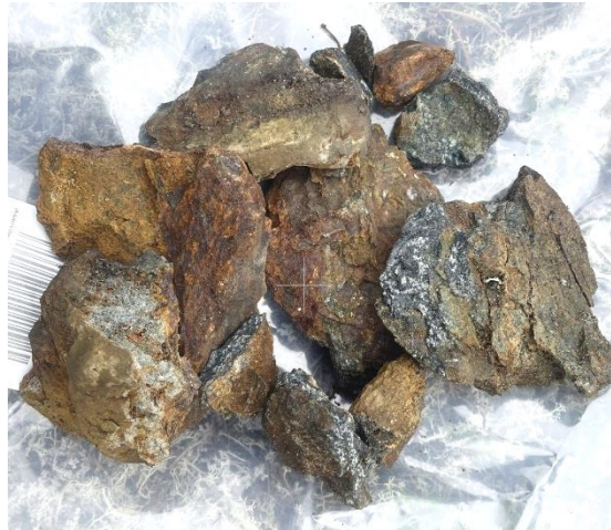
Figure 7: Photo of sample H909193 of semi-massive sulphide and gossan (20-30% oxidised pyrite and gossan) in mafic volcanic rock with assays returning 42.4 g/t Au.
