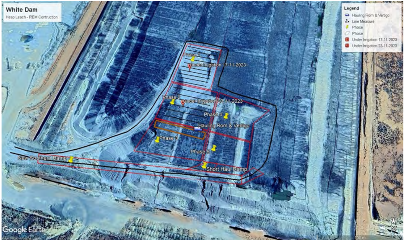
Figure 10: Aerial picture of the ROM pad with the staged 5 phases of material being restacked for cyanide irrigation.
