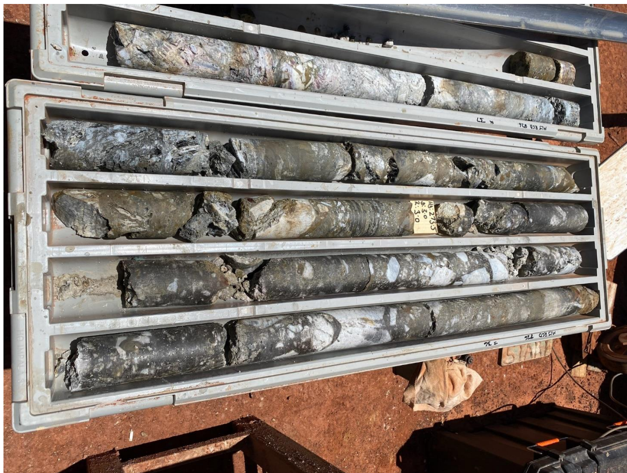
Figure 5. MLJRCD826 interval 271.6-276.0m, showing vughy silica alteration and breccia within a large 40m thick breccia zone extending from 271-311.3m, with assays pending.
