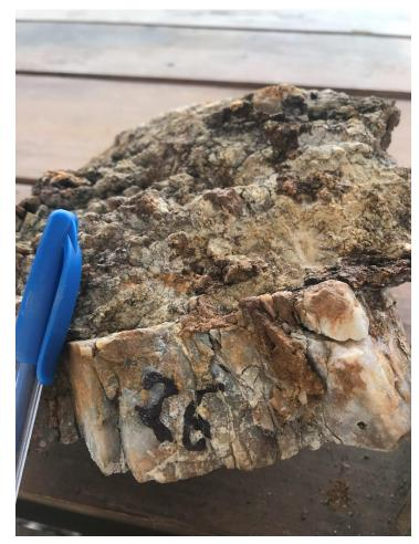
Figure 5: Weathered quartz vein with kaolinite. The kaolinite in particular is associated with the pegmatites that can host spodumene.
