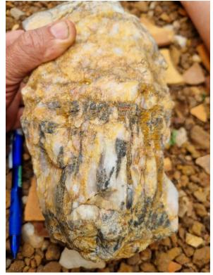
Figure 4: Coarse crystals of tourmaline with fine muscovite in a piece of quartz rich float. Such minerals are found in association with pegmatite intrusions. The softer feldspar and lithium rich spodumene are eroded or leached when near surface leaving the harder quartz and other minerals. Drilling will determine whether there is spodumene rich pegmatite at depth.
