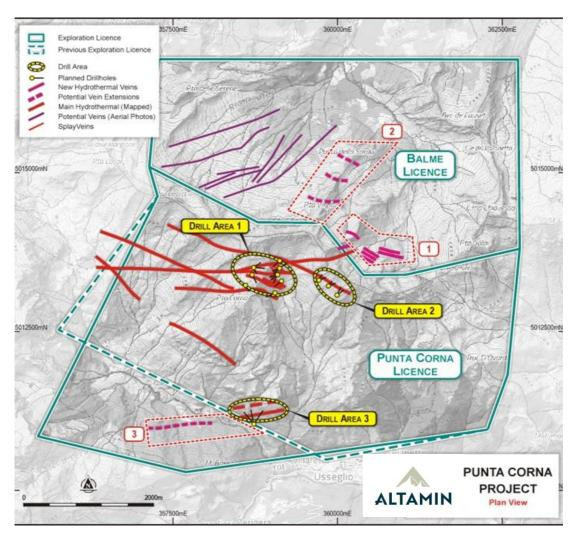
Figure 2: Punta Corna & Balme ELs showing mapped vein extensions & planned drill areas
