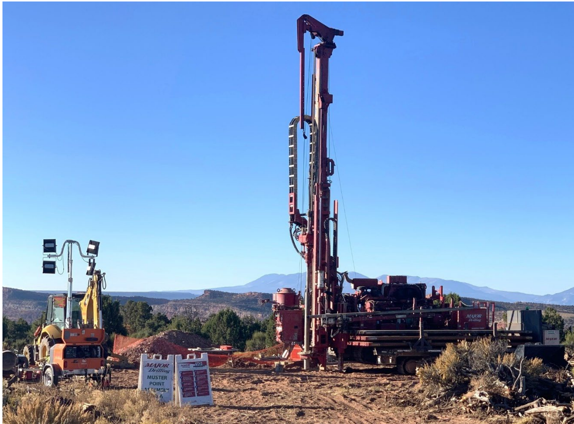
Figure 12: RC drilling at the Copper Warrior Project, Utah.
