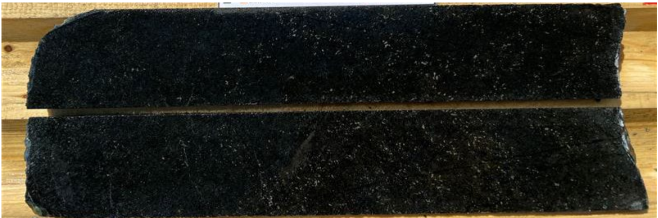
Figure 2: DDED23-131 interstitial to disseminated sulphide mineralisation
