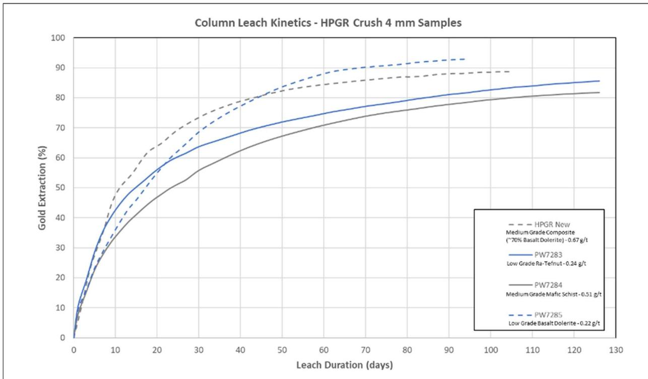
Figure 3: Column Leach Recovery Test Curves 4 mm P100 HPGR – strong leach kinetics – a predictable narrow band of recovery results.
