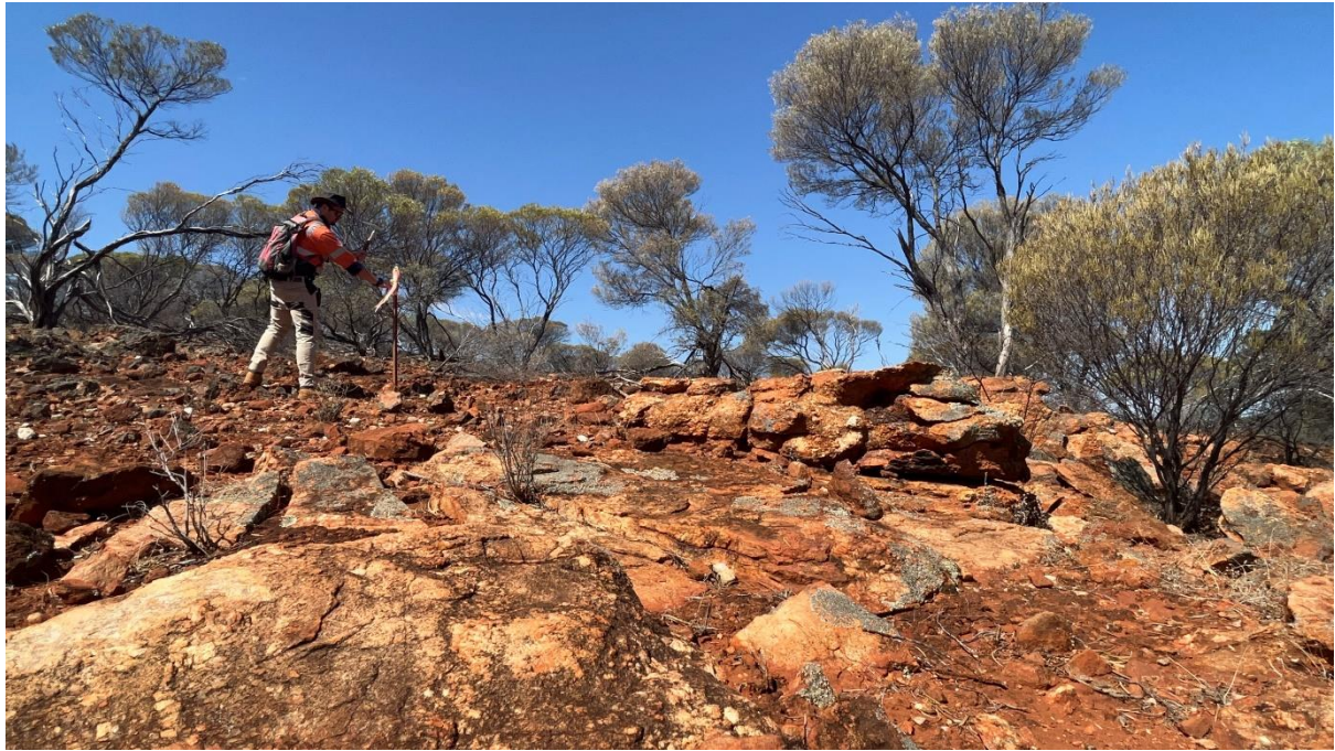
Figure 4: Pegging revised drill positions targeting outcropping pegmatite
