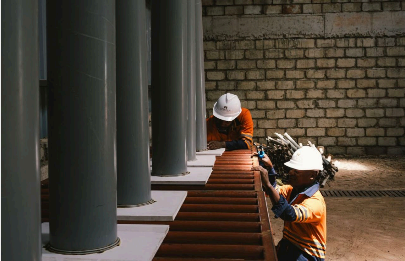
Figure 5: Inspection of constructed desorption columns.
