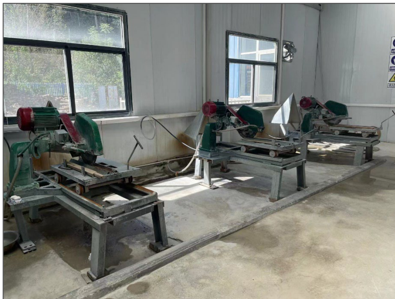
Figure 5-5: Core splitting machine at TLP
