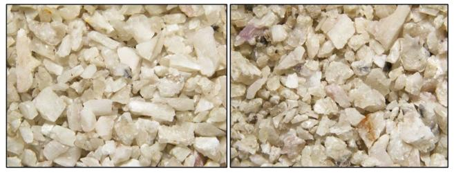
Figure 4 - HLS concentrate fractions grading ~6.0% Li<sub>2</sub>O (left) and ~5.5% Li<sub>2</sub>O (right)
