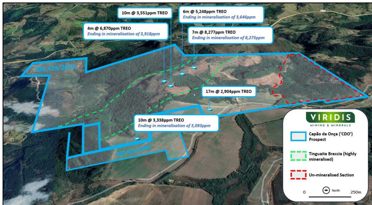
Figure 3: Satellite view of Capão da Onça, which highlights the interpreted corridor of significantly high-grade mineralisation and area of concession, which remains un-mineralised in economic levels of TREO (~<800ppm).
