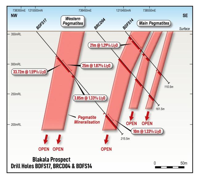
**Figure 2:** Section showing BDSF17 with the Western Pegmatite and Main Pegmatite intersected, as well as the well mineralised Series Two hole BRCD04 and the Series One hole BDSF14 on the northern extension of the Main Pegmatite body
