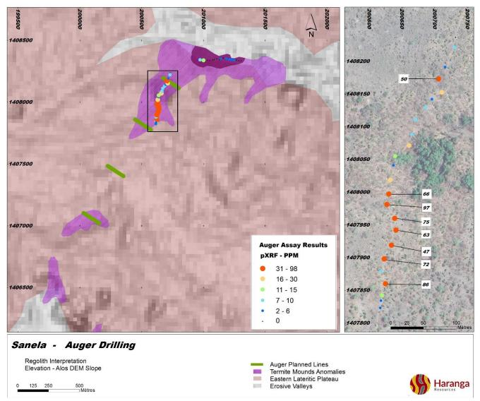
Figure 4: Location and assay results of the first auger drilled line at the Sanela Prospect<sup>3</sup>. The assay results in the saprolite below the lateritic cover range from 47ppm to 97 ppm uranium.
