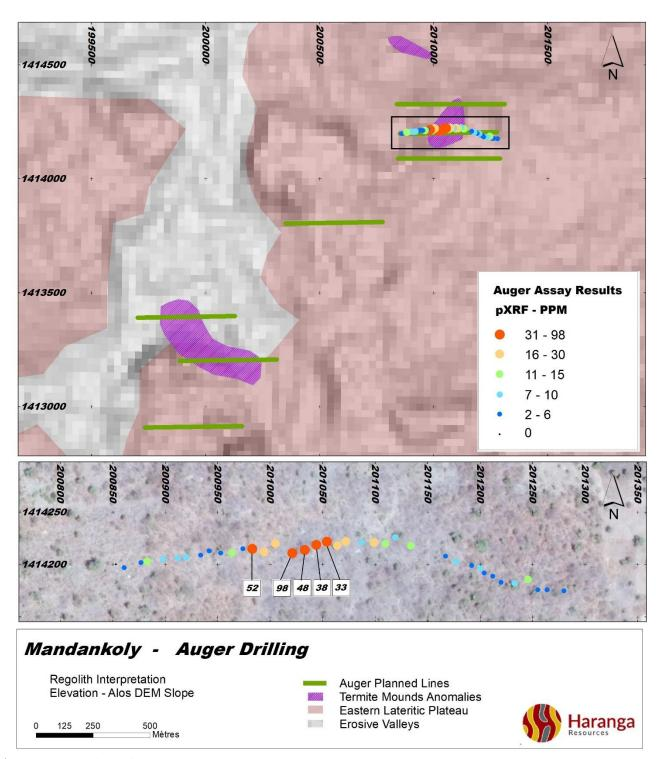
Figure 2: Location of the completed auger line at Mandankoly, over the termite mound anomaly<sup>4</sup>, and planned auger lines. Bottom window is the detail of the drilled line.
