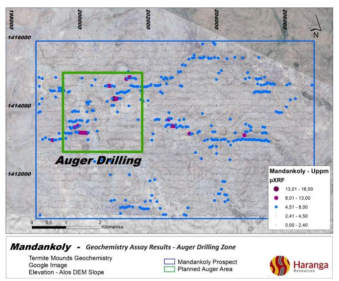
Figure 1: Location of the auger drilling zone selected from the termite mound sampling results at the Mandankoly prospect<sup>234</sup>.
