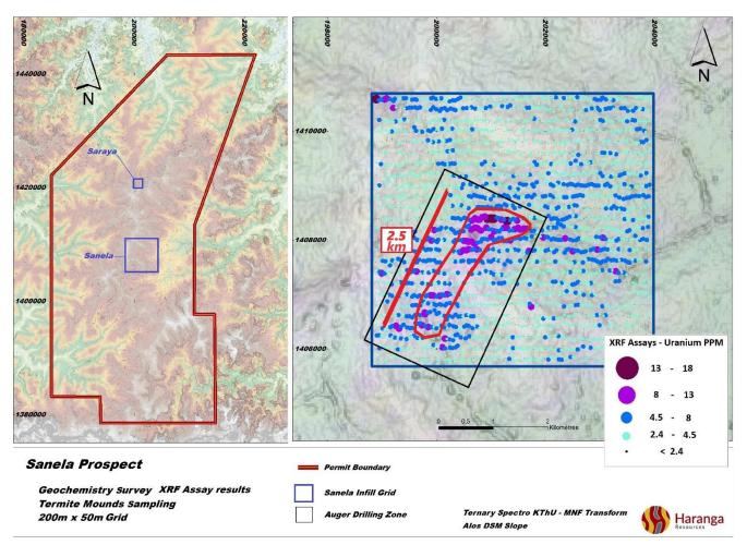
Figure 3: Location of the Sanela NNE trend with termite mound uranium concentrations and auger drilling target zone at the Sanela Prospect<sup>3</sup>.
