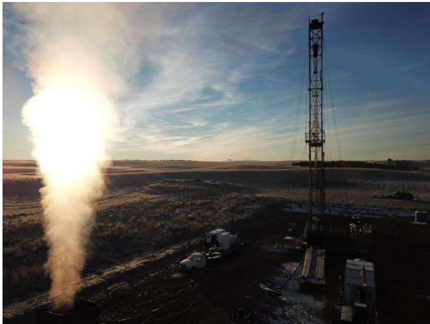
Figure 1: Jesse-1A flare-stack venting reservoir gas and helium at a rate of 1mmcf d 1
