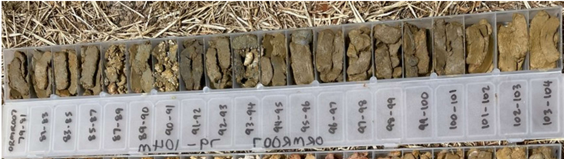
Image 2: Drill samples from ORM007 at the Rankin Rd Target showing the limonite rich fluid from 101-104m with a small uranium zone occurring at 101m. The kaolinitic clay marker bed at 85-94m.
