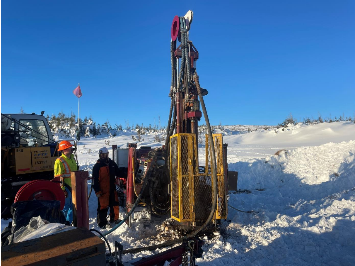
FIGURE 1: RC DRILLING AT O-2 TARGET AT MALACHITE
