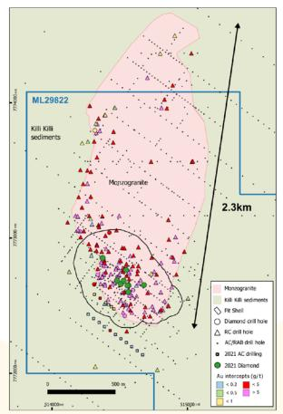
Figure 10. Buccaneer local geological map with pit shell showing maximum downhole intercepts<sup>10</sup>
