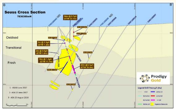
Figure 4 Cross Section of Seuss Zone showing holes HYRC2305 and HYRC2350A<sup>3</sup>
