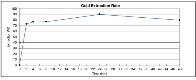
Figure 4: Leach Recovery Test Curve – Rougher Flotation Tailing
