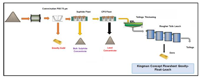
Figure 5: Gravity-Flotation-Leach Concept Flowsheet Tested
