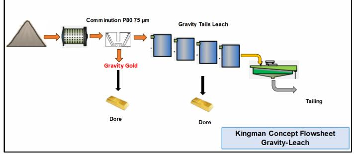
Figure 3: Gravity-Leach Flowsheet Tested
