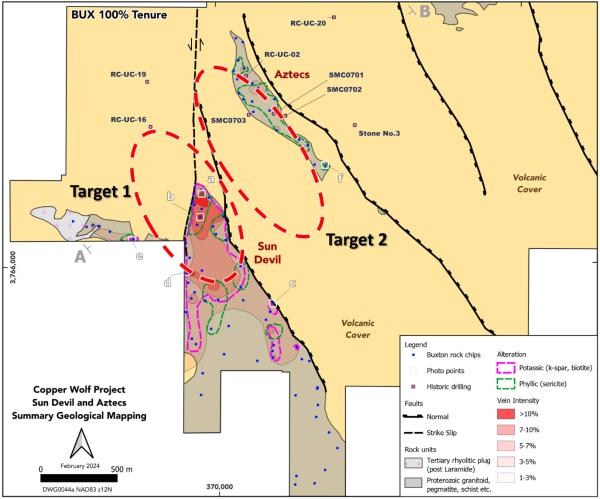
**Figure 1:** Buxton's mapping & chip sampling at Sun Devil and Aztecs prospects with mapped vein intensity & alteration limits. Figure 2 is a cross section along line A-B.
