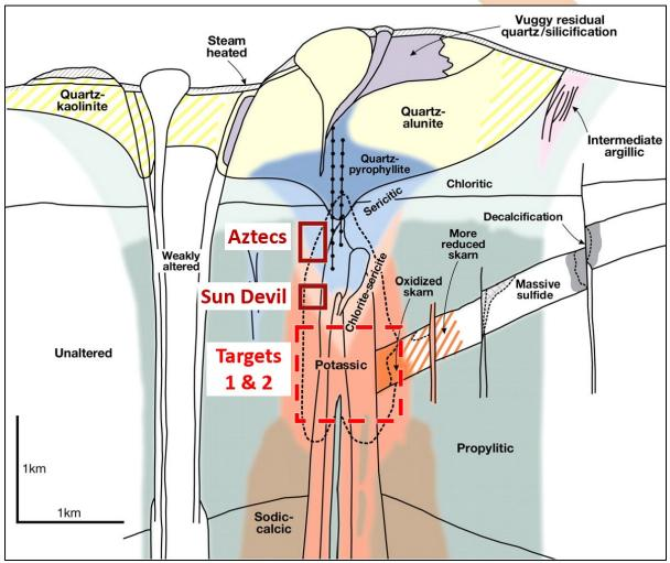
**Figure 4:** Schematic ross section showing generalised alteration-mineralization zoning patterns for porphyry Cu deposits by Sillitoe (2010). The chlorite-sericite alteration zone is not typically found in Cu-Mo systems, which are dominantly sericitic. The interpreted positions of the Sun Devil and Aztecs prior to tilting & faulting of the Copper Wolf West porphyry system are annotated. Oxidiation and supergene enrichemnt will overprint these alteration relationships.
