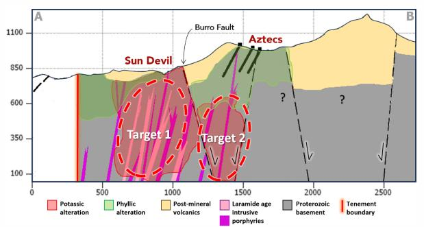
**Figure 2:** Interpretive geological cross section looking northwest through the western Copper Wolf Project area. Two target zones of potassic alteration are shown at depth. These are likely to have been part of the same porphyry system that has been dissected by the Burro Fault.
