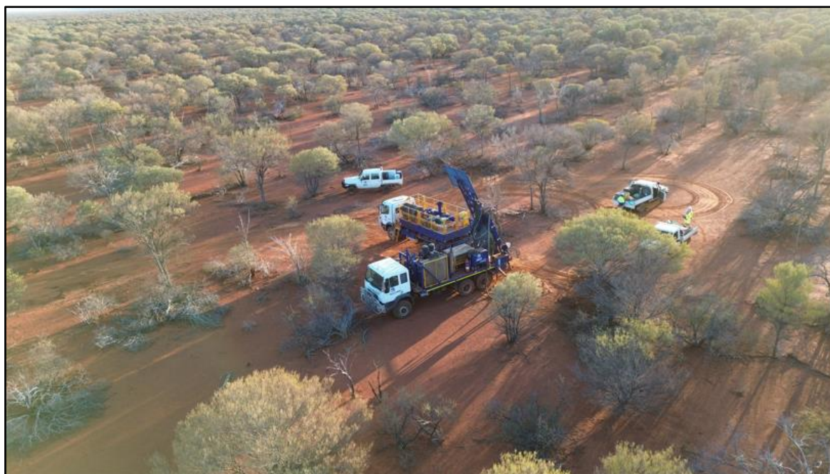
Figure 6: Aircore geochemical drilling in typical soil-covered terrain at the Yarri Project. Extensive soil cover means that any previous surface geochemical sampling can be considered to be largely ineffective.
