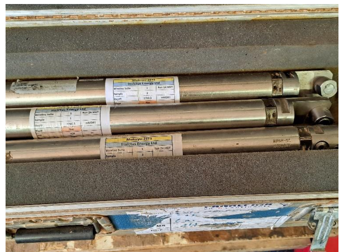
Figure 1 - Downhole gas samples recovered to surface in pressurised chambers in preparation for shipment to the lab for analysis
