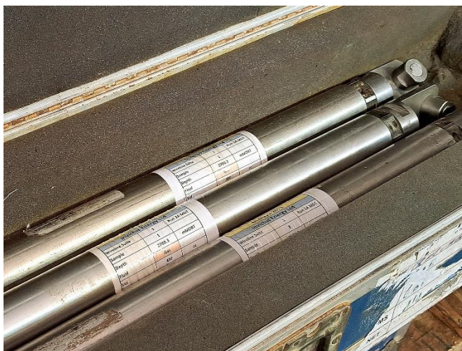
Figure 1 - Downhole gas samples recovered to surface in pressurised chambers in preparation for shipment to the lab for analysis
