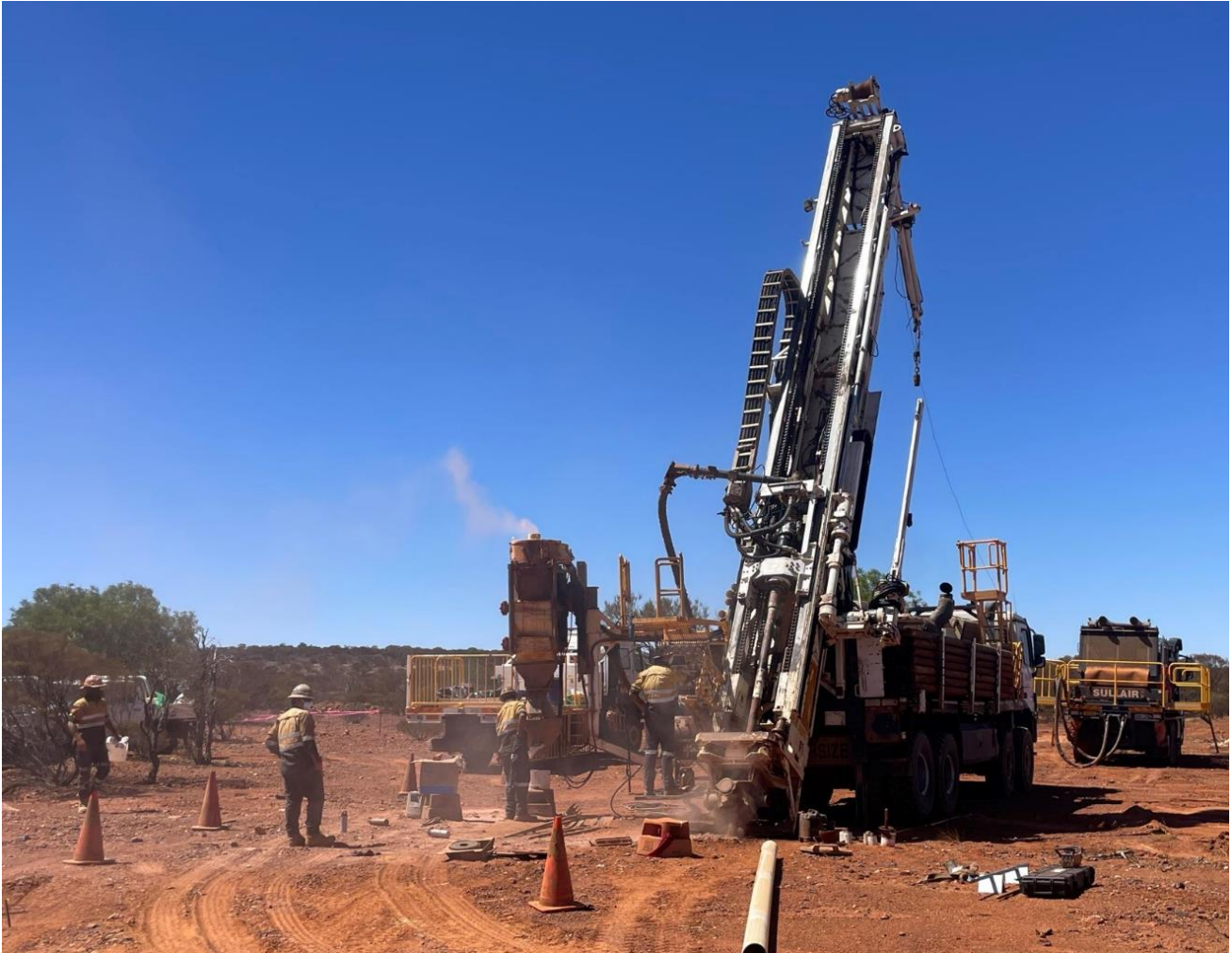
Figure 1 - RC drilling underway at the T8 Target on the Tuckanarra Project
