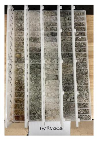
Figure 3: RC drill hole INRC08 - 20m white quartz intersection 35m to 55m
