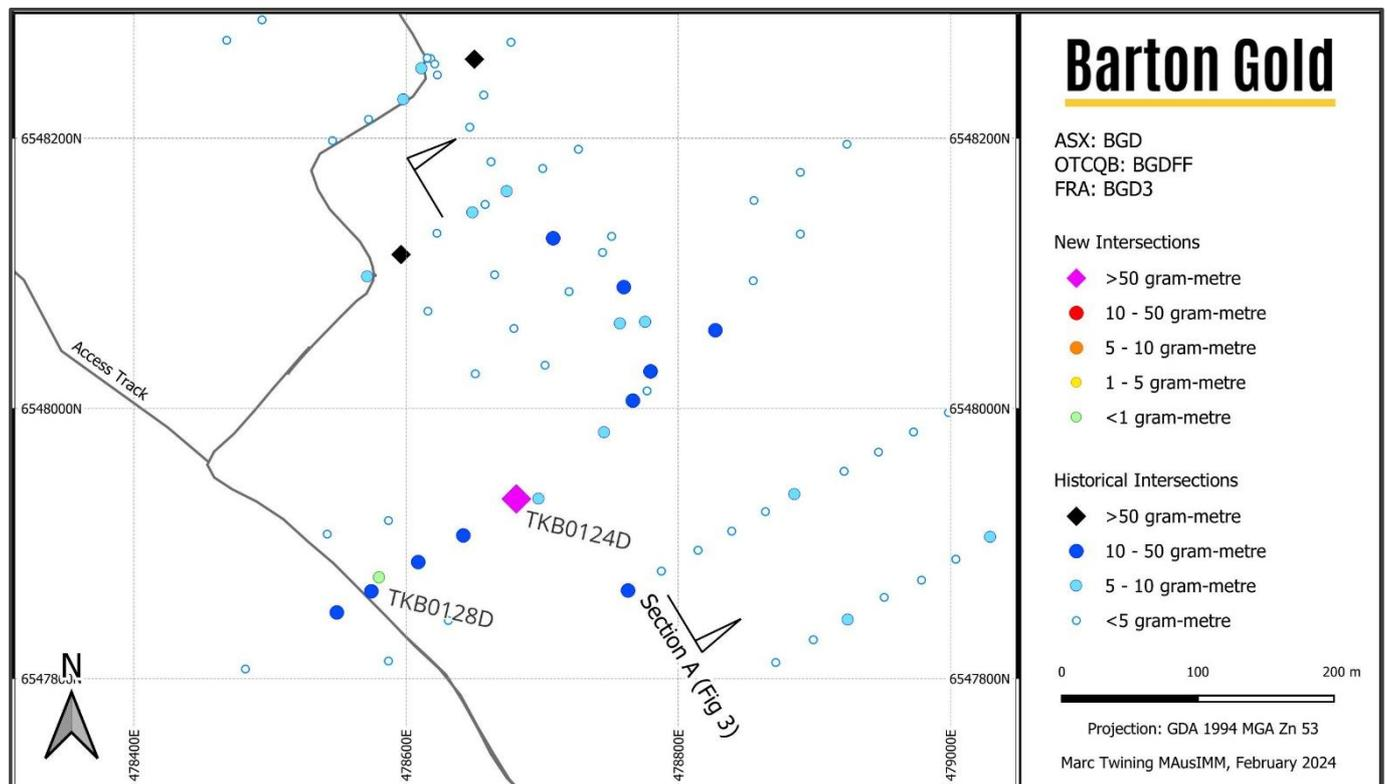
**Figure 2 – Tunkillia Area 191 drilling plan showing new and historical drill hole collars**
