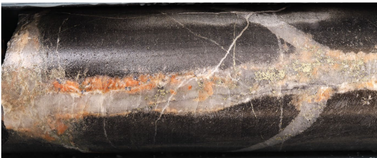
Figure 4 Mineralised volcanic sediments in 23BRD0024, 167.3m depth from a 2m sample which assayed 0.4% Cu and 197ppm Mo. Core diameter 61.5mm.
