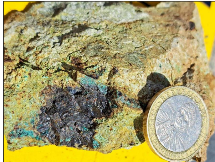
Sample # 8615 grading 5.37% Cu from the Lucero Prospect (ASX announcement 21 November 2023).
