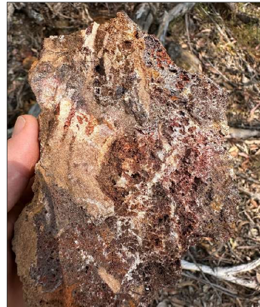
Figure 4 – Gold-Silver-Lead mineralisation within ferruginous quartz-schist yielding 3.16 g/t Au 9.25 g/t Ag from sample 300185
