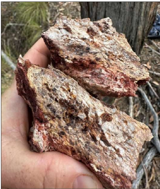
Figure 3 – Gold-Silver-Lead mineralisation within ferruginous quartz-schist yielding 0.62 g/t Au 85.25 g/t Ag & 0.35% Pb from sample 300218
