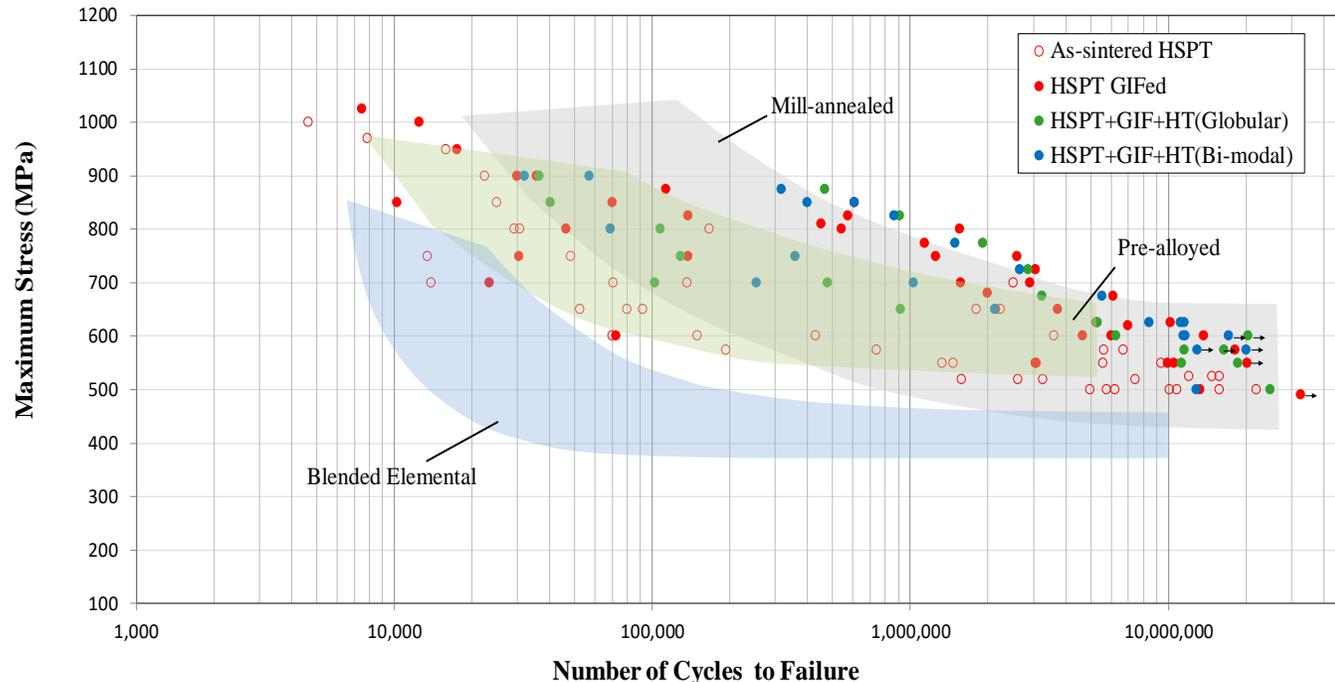
HSPT = Hydrogen sintering and Phase Transformation; GIF = Gaseous Isostatic Forging; HT = Heat Treatment
