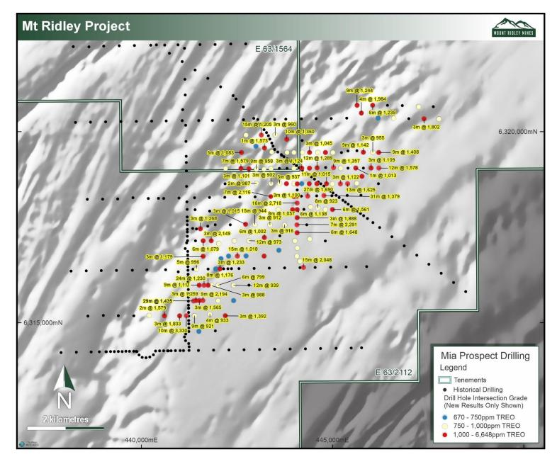
Figure 2: Infill drill holes demonstrate that highly enriched REE mineralisation is often continuous between earlier drill holes. Mineralisation often occurs along linear, magnetic 'ridges' seen in aeromagnetic imagery. Red dots are significant intersections with an average grade >1000ppm TREO (using a 700ppm TREO lower cut) from the October 2023 drilling programme.
