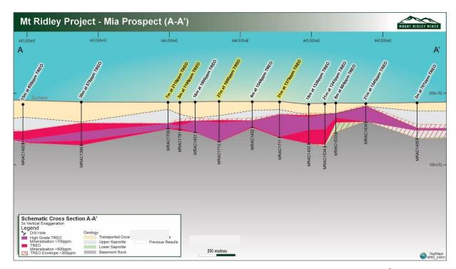
**Figure 3:** East-west **c**ross section across the Mia Prospect at approximately 6,318,300mN, (see Figure 6 for location). High-grade mineralisation is approximately 1.4km wide. October 2023 holes are shown with yellow highlight. The vertical scale is 5x the horizontal scale.
