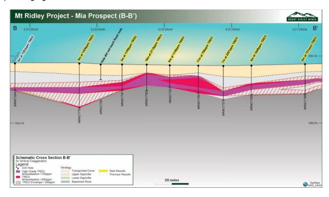
**Figure 4:** North-south section along the Mia Prospect at approximately 444,070mE, (see Figure 6 for location). High-grade mineralisation has an oblique width exceeding lkm. October 2023 holes are shown with yellow highlight. The vertical scale is 5x the horizontal scale.
