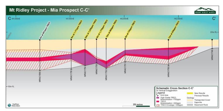
**Figure 5:** Cross section across the Mia Prospect at approximately 6,315,980mN, (see Figure 6 for location). The thick zone of high grade clay-hosted REE mineralisation is approximately 300m wide. Key drill holes are 100m apart. New holes are shown with yellow highlight. The vertical scale is 5x the horizontal scale.
