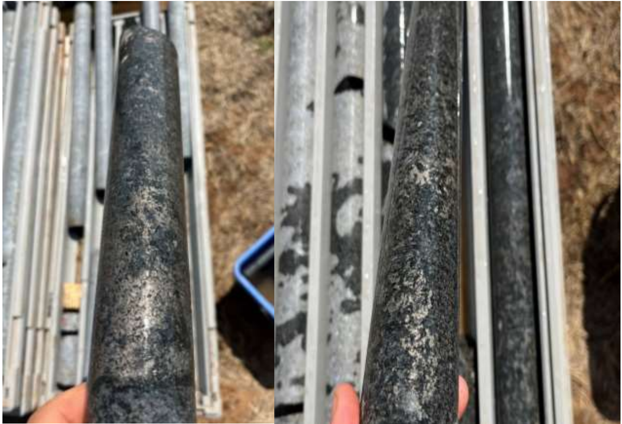
Figure 3. Photos showing examples disseminated and blebby sulphides in hole BRDD002. (Left) Nickel-Copper sulphides at 348m, (Right) Disseminated sulphides 338 – 342m Note core is NQ2 being 2 inches or 50mm in diameter
