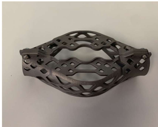
Titanium Printing Using Generative Designs
