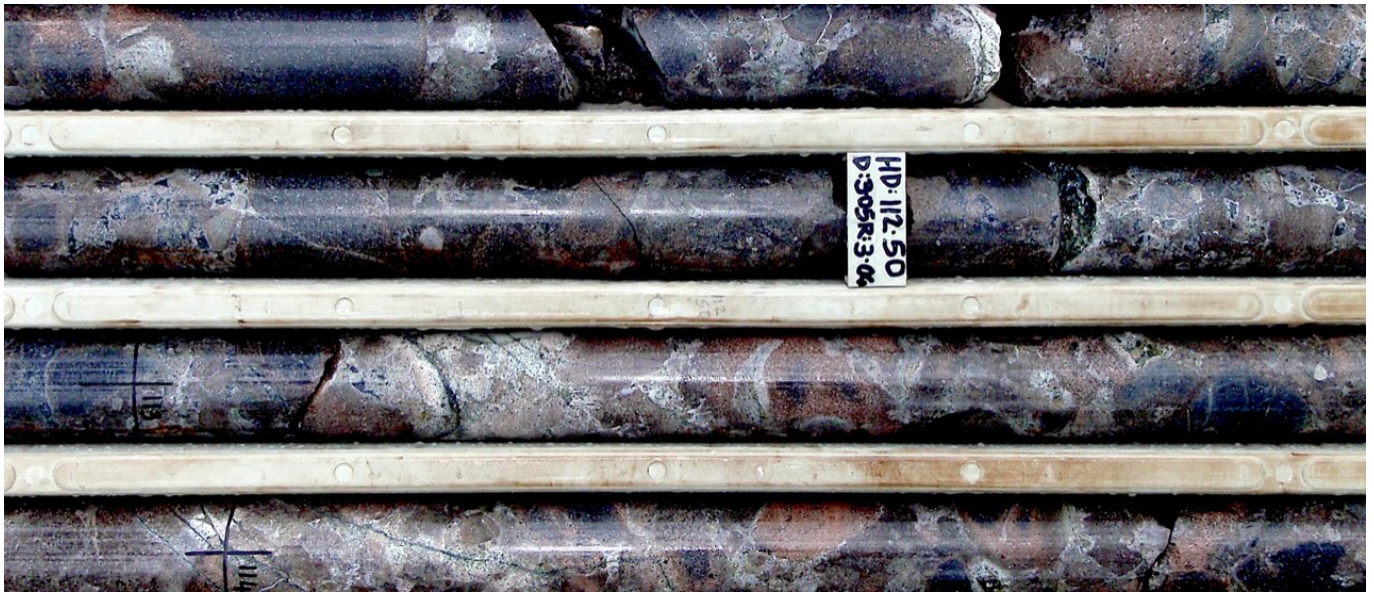
Figure 2 – Close up core photo from previous drill hole SBDD0003 (Geopacific HQ, 111.2m to 114.70m) illustrating jigsaw crackle breccia, clast supported with infill of quartz and sulphides.
