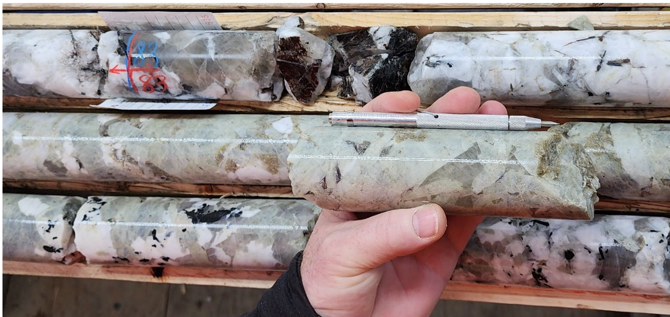
Figure 1: Up to 70% estimated spodumene mineralisation over 3.3m in DDH1557-24-041.
