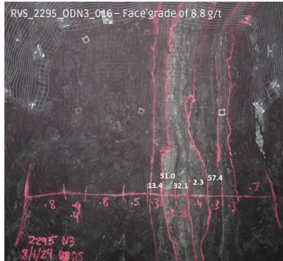
Figure 1 – 2295 N3 drive showing face samples and average cut grade
