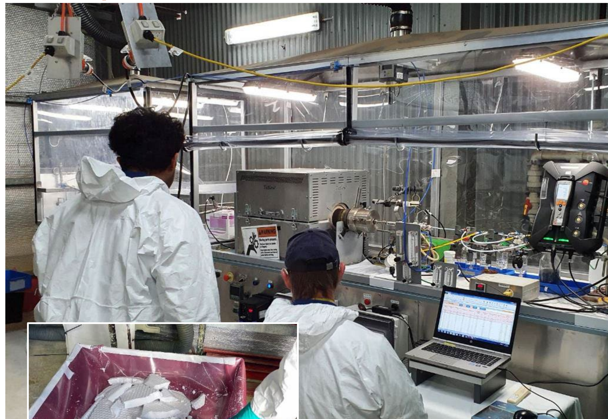
Above: Goschen's rare earth product undergoing bench scale sulphation kiln testwork at ANSTO.
