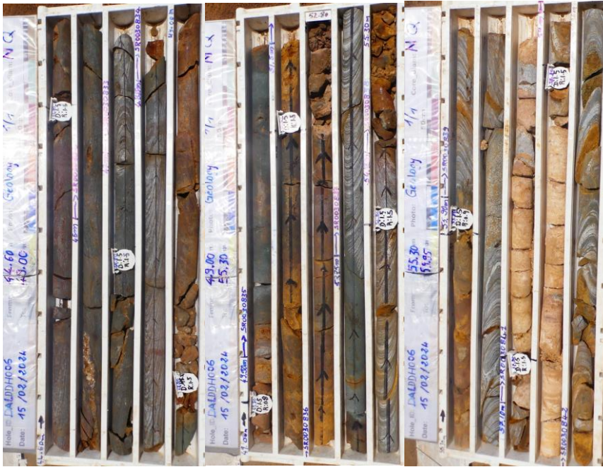
Figure 9: DALDDH006 photographed core which includes iron oxide intervals from Table 1
