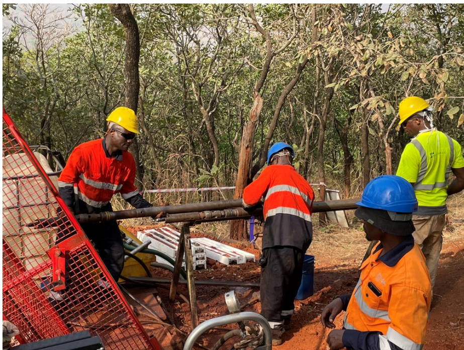
Figure 7: Energold drill crew in process of recovering drill core from the core barrel on drill hole DALDDH0011 at Dalabatini Prospect
