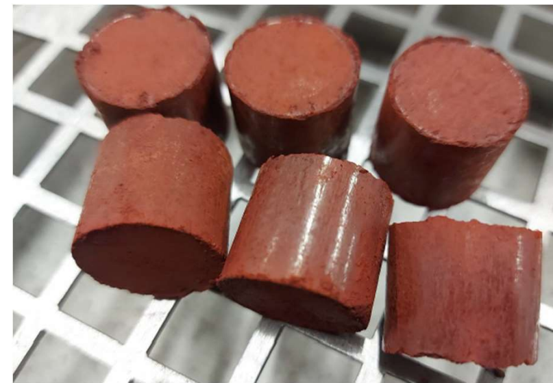
Figure 2 - Cylindrical Test Specimen (CTS) pellets produced from red mud iron samples.
