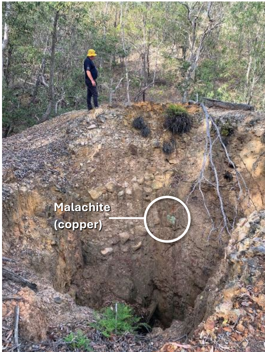
Figure 10. New shaft Identified 620m south-east of the old workings. Visible malachite in the wall of the shaft, with vertical depth of shaft estimated at 60m.
