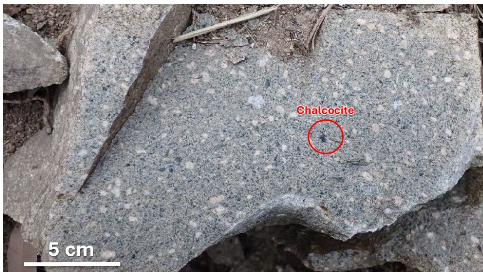
Figure 12. Specimen sample from the field of porphyry andesite containing chalcocite at Kaa prospect.
