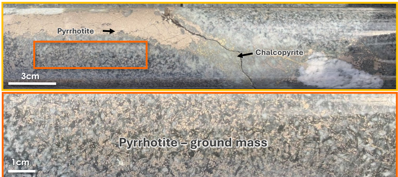
Figure 17. Texture of the semi-massive sulphides, dominantly pyrrhotite and chalcopyrite within magmatic unit, cumulate texture within diamond core, Fox Prospect - Tanami.
