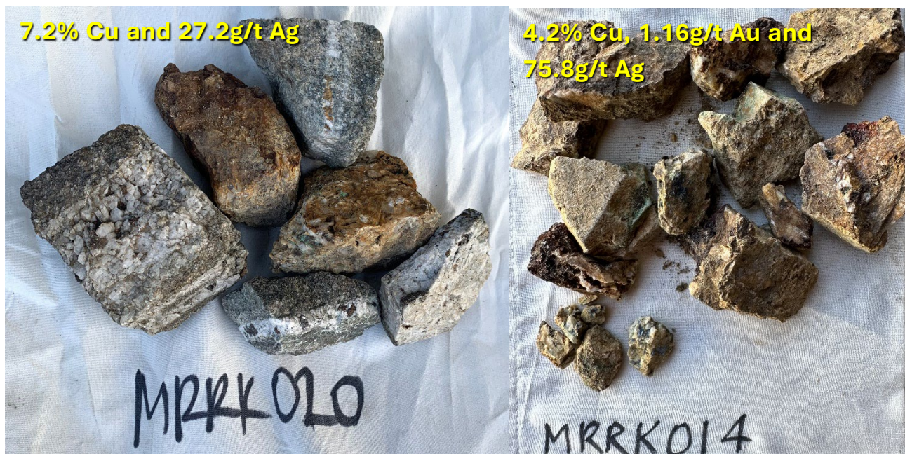
Figure 4. Rock chip sample MRRK020, bornite crystals, 1 cm x 0.5cm in size, within quartz veins, at the contact between a mafic and a granite unit. MRRK014, iron rich quartz vein at surface.
