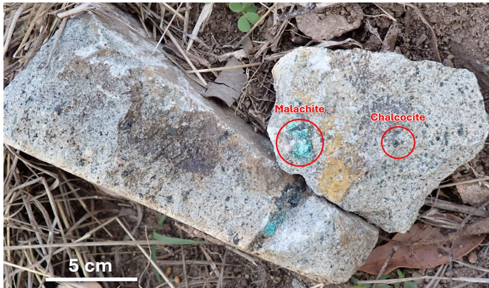
Figure 11. Specimen sample from the field of sub-porphyrific andesite, containing malachite and chalcocite blebs, from Kaa prospect.
