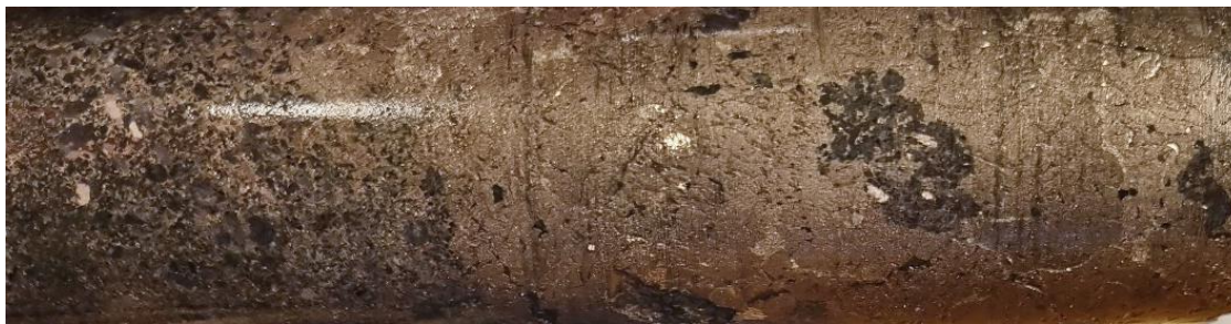
Massive and net-textured pyrrhotite-pentlandite-chalcopyrite with coarse pentlandite loop textures and rounded clasts of peridotite, from a 0.3 m sample that returned 1.71% Ni, 0.26% Cu, 0.15% Co, 176.54 m, 23RAN002. NQ diameter drill core.
