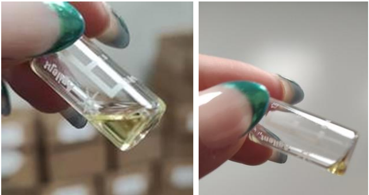
Figure 1 - Condensate recovered from flashed downhole reservoir fluid samples from Mukuyu-2 / ST11 well from Upper Angwa (on left) and Lower Angwa formations (on right) with API gravity of 50-60
