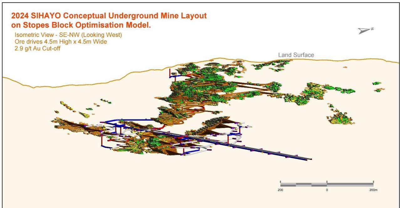
**Figure 5: Sihayo Concept Study underground mine layout (Isometric view looking W) and Stope Block Optimisation Model at 2.9 g/t Au cut-off**
