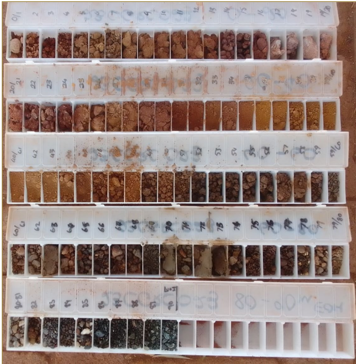
Figure 4: General styles of mineralisation encountered at Coggia seen in RC chips of laterite style (red/rust colour) through to deeper ultramafic hosted style mineralisation (blue/grey colour) at the end of the hole.
