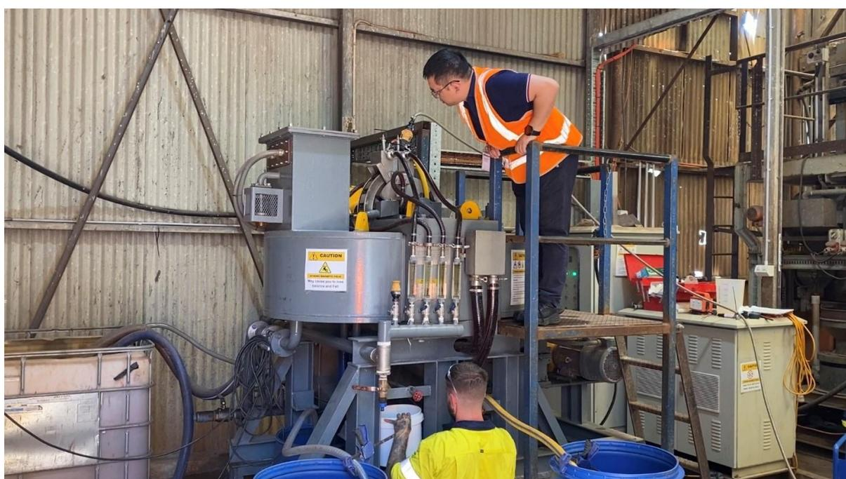
Image 3: Pilot-scale WHIMS Testing at Nagrom Laboratory in Perth, Australia
