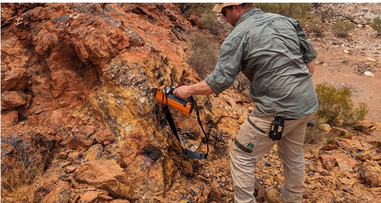
Figure 1: Photo of Dreadnought's Matt Crowe taking scintillometer readings at the historical Monster uranium target.
