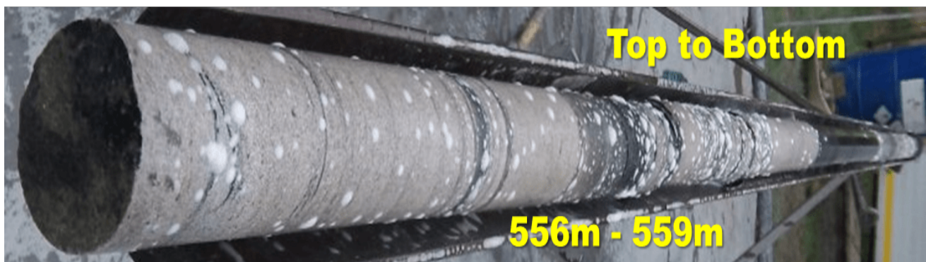
Figure 9. Three metre core run from 556-559m with gassy sandstone and dark carbonaceous zones below coal zones.
