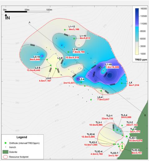
Drillhole Location Map on Trench Sampling TREO Contours
