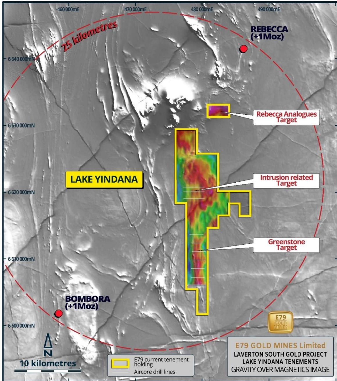
Figure 3: Map of Lake Yindana with gravity over magnetics. White lines are recent aircore drill lines.
