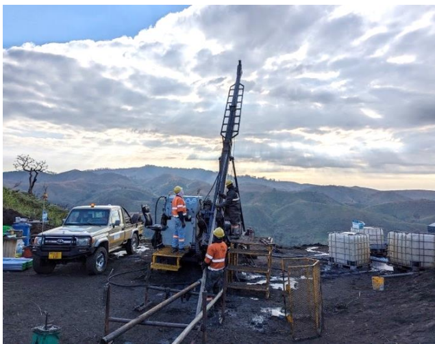
Figure 9 - Diamond Drilling on the Epanko Western Zone
